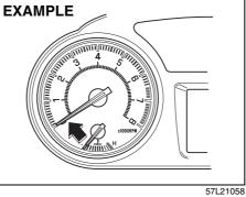
The tachometer indicates engine speed in revolutions per minute.
